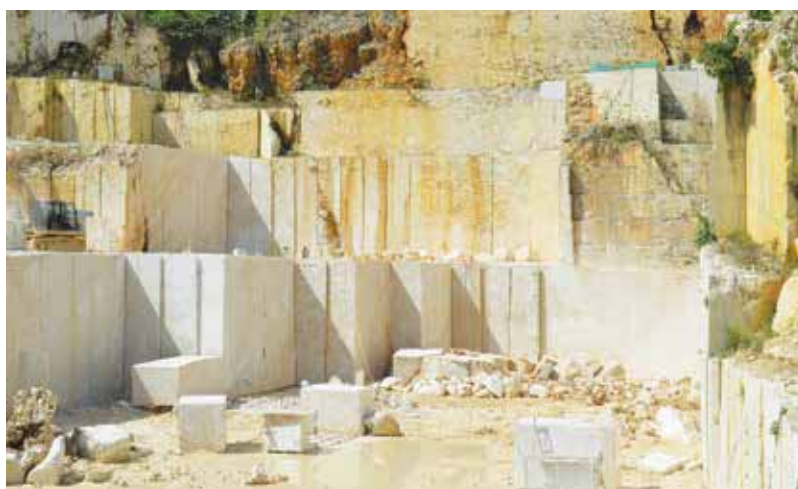
Limestone block extraction
